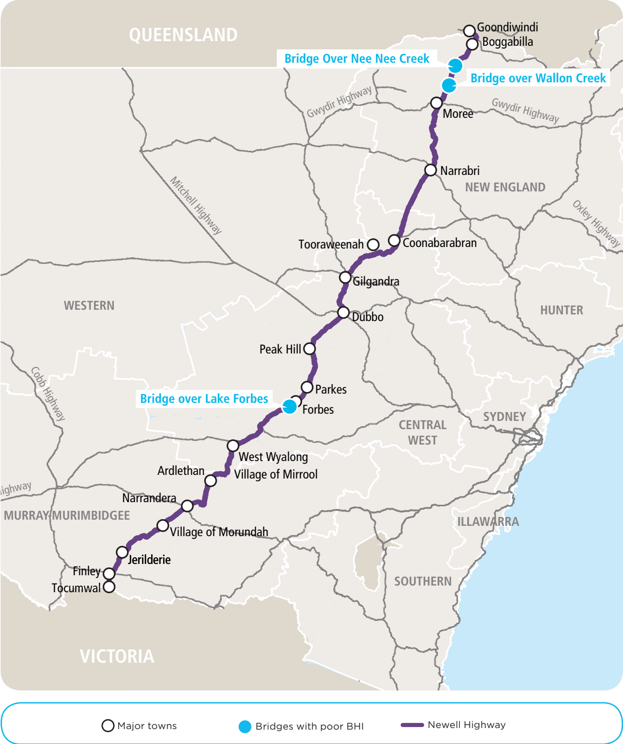
Figure 4.21 Locations of bridges with poor Bridge Health Index (BHI)
