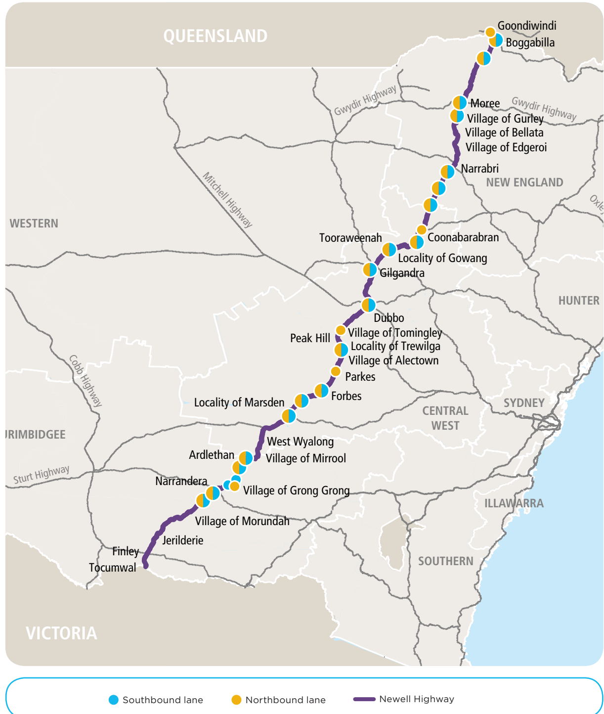
Figure 4.19 Locations where lane widths are less than 3.25 metres
