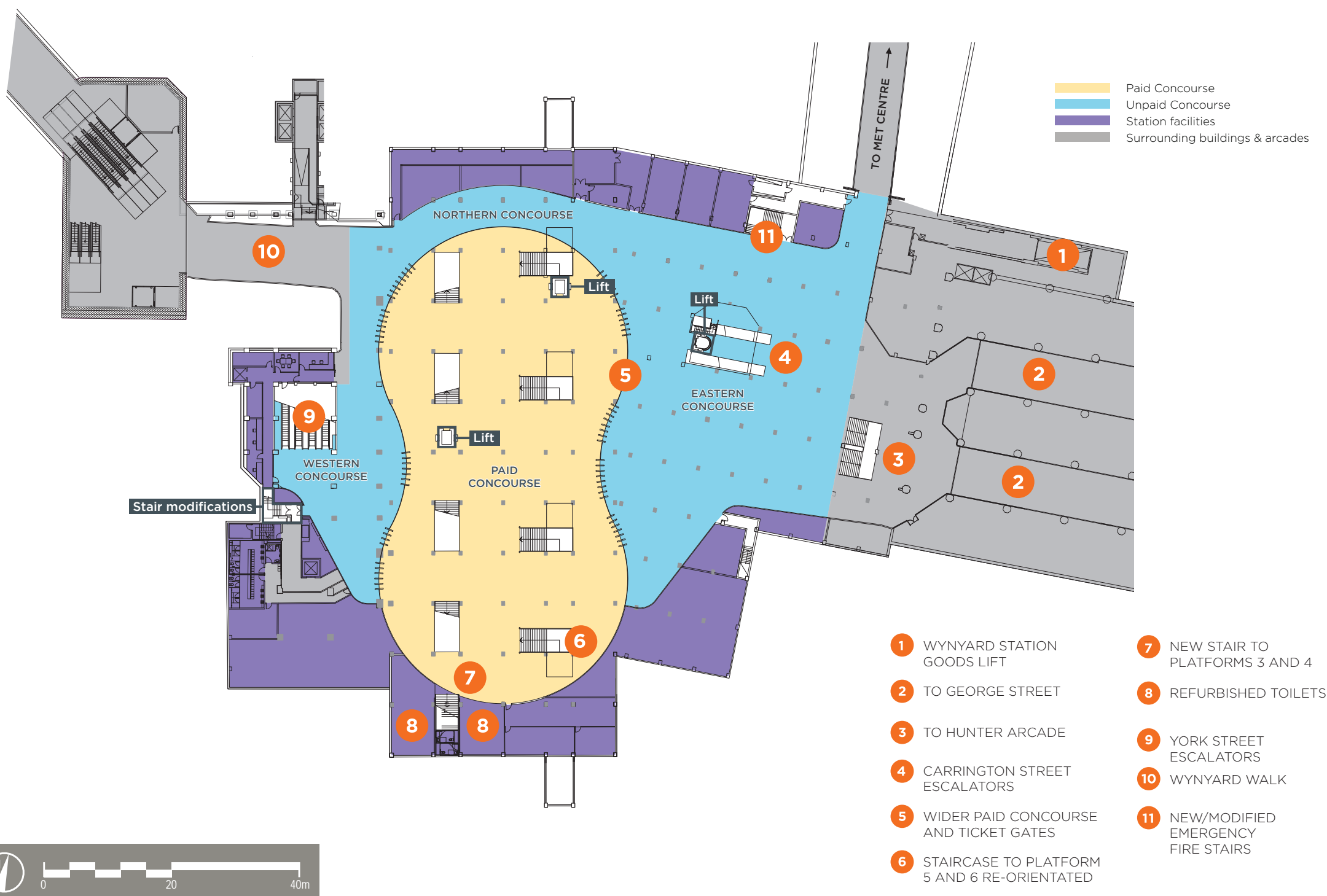
Figure 5 - Proposed Wynyard Station - concourse layout (indicative)
