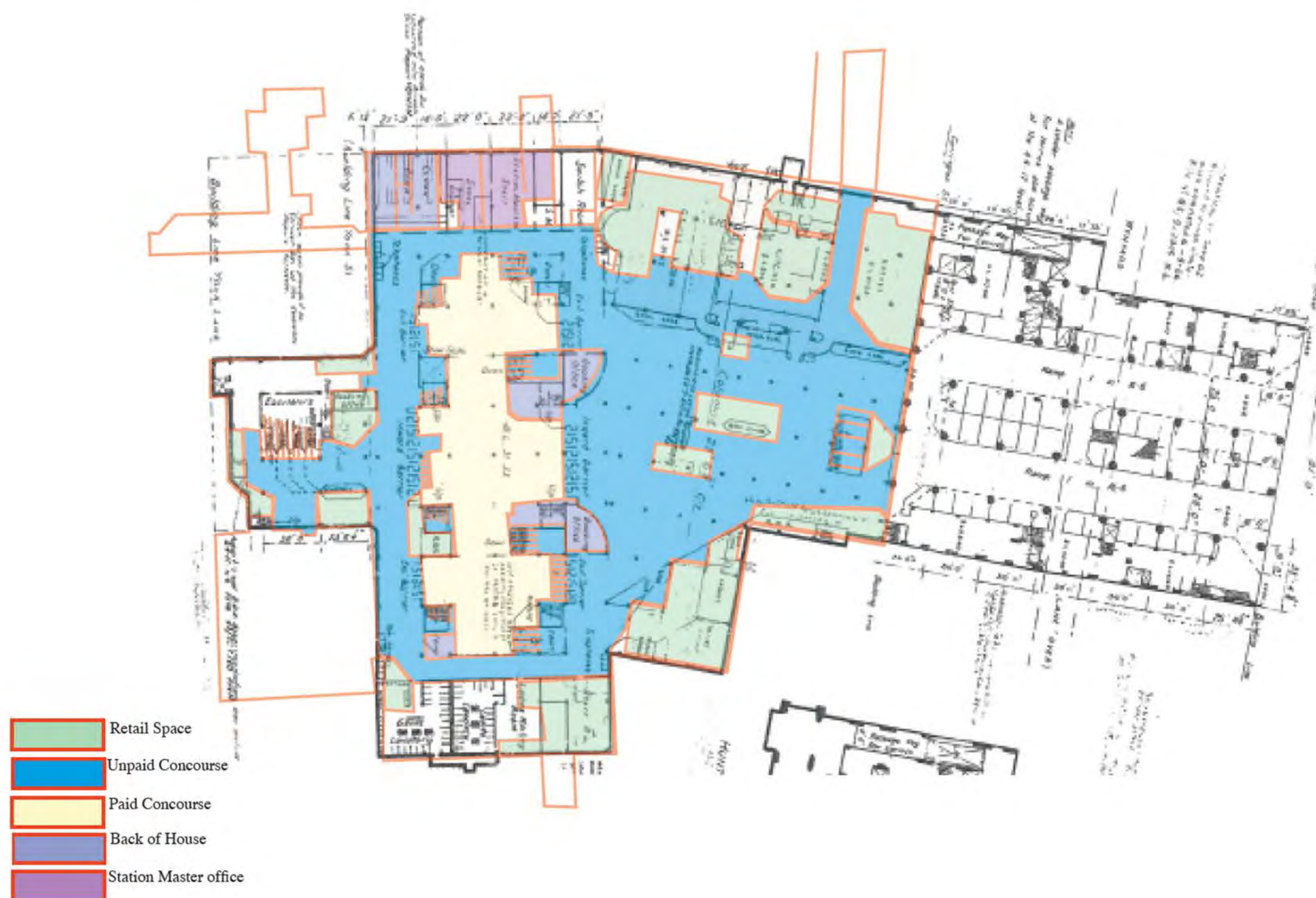
Figure 30 – Representation of the current layout of Wynyard Station (in colour) over a black and white hand-drawn base plan of the original Wynyard Station layout from the 1920s. The areas coloured in blue is the present extent of the UNPAID concourses throughout Wynyard Station. The areas coloured in yellow is the present extent of the PAID concourses. Areas in green are current retail spaces, and areas coloured in purple are Station facilities and back-of-house areas. The uncoloured areas are outside of the scope of works. Note that most of the basement levels of Transport House (north and south of the escalators in the western concourse) was undeveloped as part of the original Wynyard Station layout. (Image Source: Futurepast 26/08/2014)
