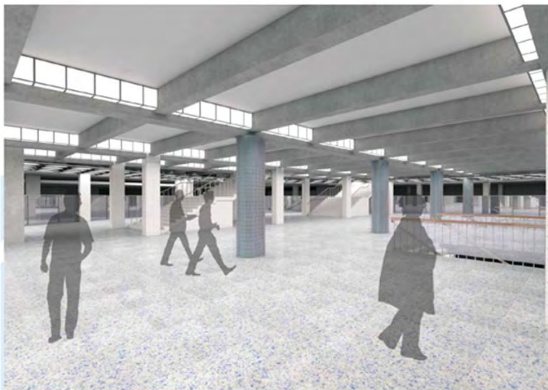
Figure 83 – Artists impression of the new refurbishment for the Paid Concourse. The existing suspended ceiling is to be removed to expose the original crossbeam ceiling. (Source: Wynyard Station Upgrade, Station Working Group Presentation 09 October 2014, prepared for TfNSW by Cox Richardson Architects)
