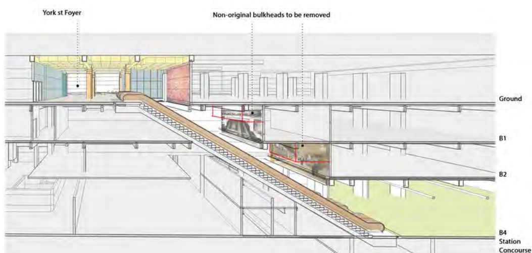
Figure 91 – Cross section of Transport House looking east, showing each of the basement levels down to Concourse Level (B4). The red line shows where the existing non-original bulkheads would be removed in front of a new glazed one-way viewing window, with opportunity to use it as a heritage interpretation panel. (Source: Pers. Comms. Caitlin Bennett 10/11/14)
