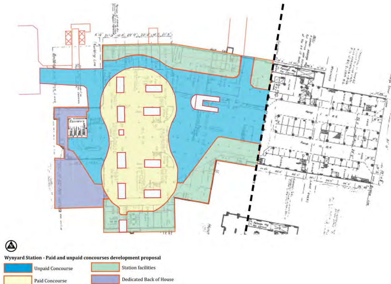
Figure 63 – The proposed works overlaid over the original layout of Wynyard Station (Source: Futurepast 20/10/2014)
