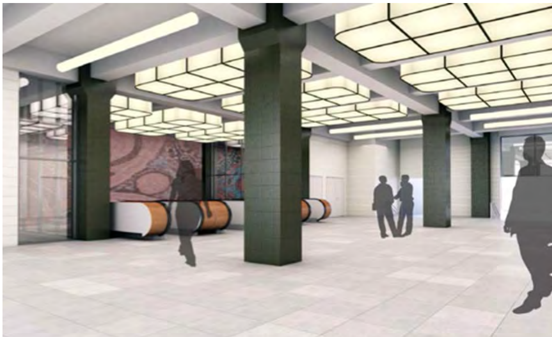
Figure 87 – Artists impression of the new refurbishment for the York Street Foyer, with new floor, wall and column cladding. The original cross-beam ceiling is to be exposed, with new art-deco style box lights to be positioned in between the cross-beams. (Source: Wynyard Station Upgrade, Station Working Group Presentation 09 October 2014, prepared for TfNSW by Cox Richardson Architects)
