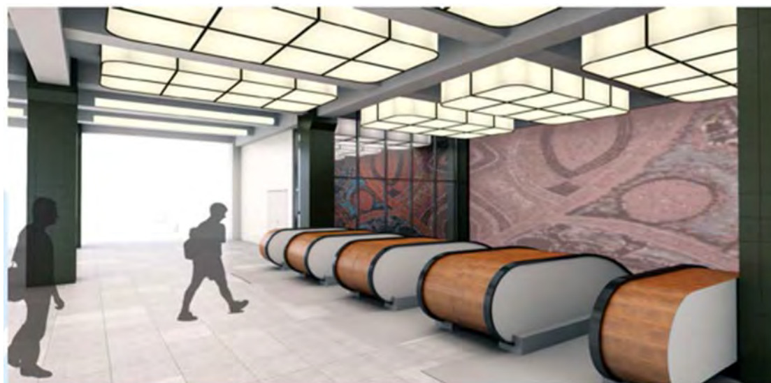
Figure 88 – Artists impression of the new refurbishment for the York Street Foyer, with new floor, wall and column cladding. The original crossbeam ceiling is to be exposed, with new art-deco style box lights to be positioned in between the cross-beams. (Source: Wynyard Station Upgrade, Station Working Group Presentation 09 October 2014, prepared for TfNSW by Cox Richardson Architects)
