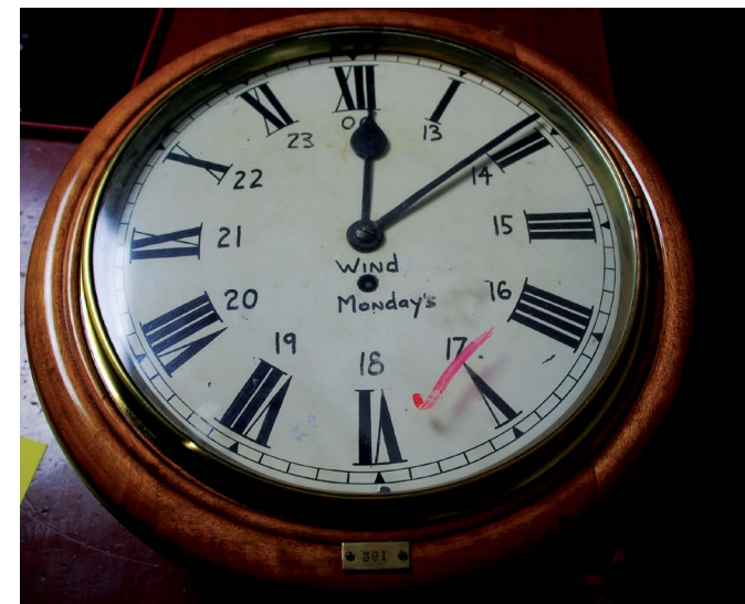
Figure 46: An example of a round-faced, English clock used extensively in the NSW railways network. Unlike Seth Thomas clocks, these clocks ran on an internal fusee system which ran for 7-8 days before it needed winding. This clock has a number of individual modifications including the addition of 24-hour time markers on the face and the reminder to wind it Mondays. Note the identification number on the brass plate at the bottom (Source: Sydney Trains)
