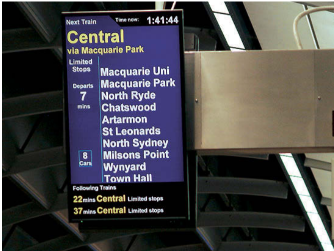
Figure 38: An example of the first generation of electronic platform information boards at Epping with the actual time and departure times visible on the screen (Source: Sydney Trains)
