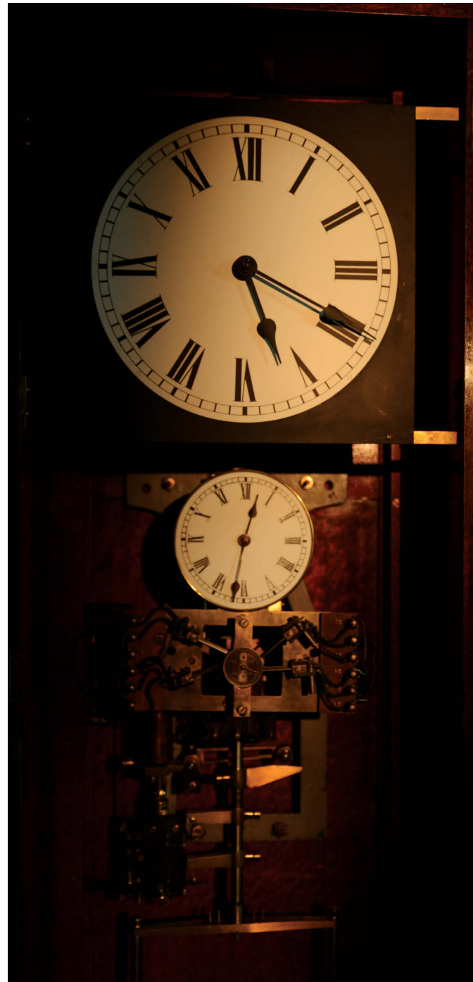
Figure 33: A 'Timatic' master clock, the same as was originally installed at Prince Alfred Sidings, Central station, as well as at Transport House and other master clock locations. Two such master clocks (thought to be from Central) are now held in the historic clock collection of Sydney Trains (Source: Sydney Trains)
