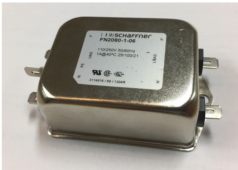
Figure 38 - 120/24V Schaffner LEU Power Supply Filter Module
