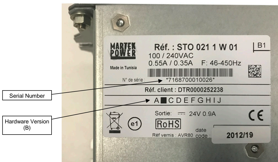
Figure 37 - MIPS200 Power Supply Serial Number and Hardware Version
