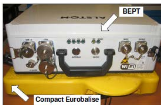
Figure 71 - Placement of BEPT on to balise
