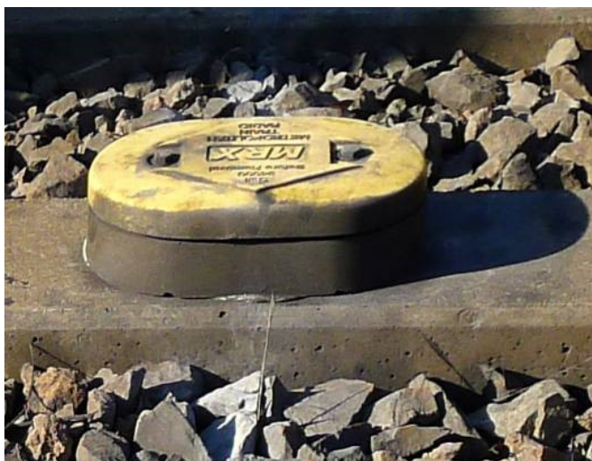
Figure 4 - Metronet Transponder with Base Glued to a Concrete Sleeper
