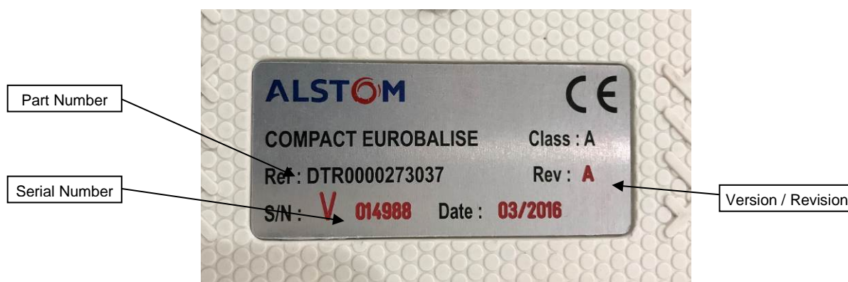
Figure 2 - Identification of Balise Serial Number and Version (Revision)
