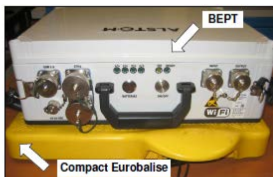
Figure 70 - Placement of BEPT on to balise
