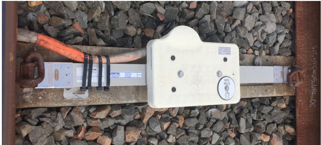
Figure 6 - Balise Mounted on a Vortok eClip Beam
