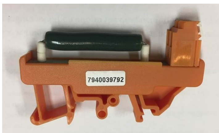
Figure 30 - Detail of 150 Ohm Resistor Module
