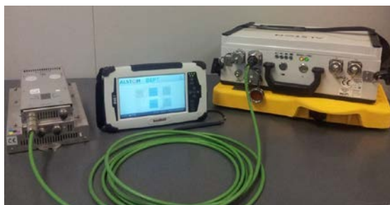
Figure 78 - Connecting BEPT to Ethernet Port 1 of LEU
