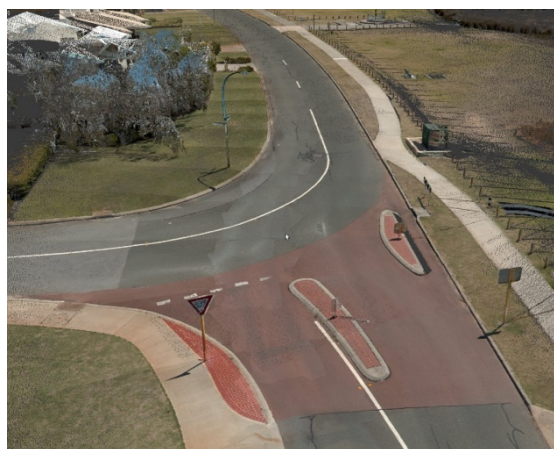
Figure 15 LiDAR point cloud representation of local government road (Source: Anditi)
