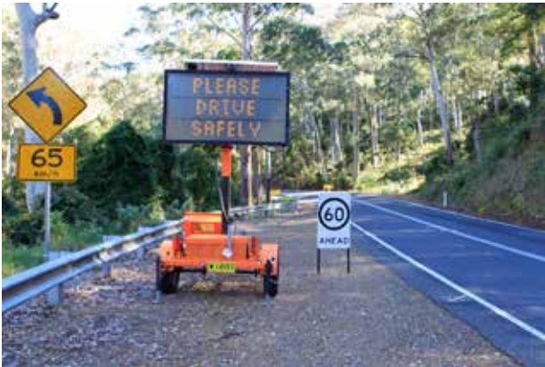
Photograph 3.8: Portable variable message sign within the clear zone
