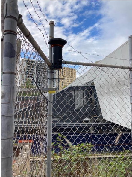
Photo 14 – Noise monitors installed on LES compound and near Marian Street compound.
