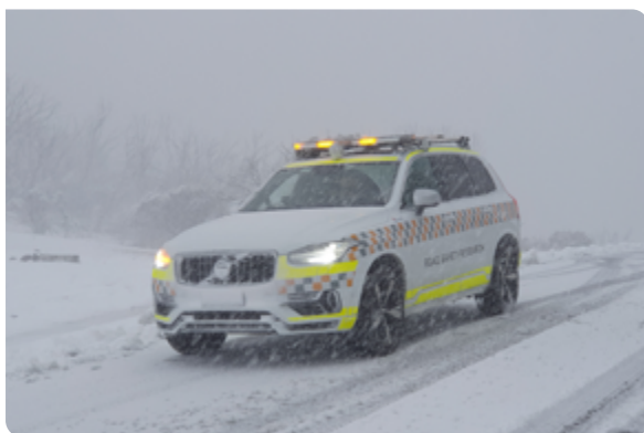
The highly automated research vehicle (SAFETI) assessing the capability of the vehicle's Lane Keep Assist and Traffic Sign Recognition systems in the Snowy Mountains.
