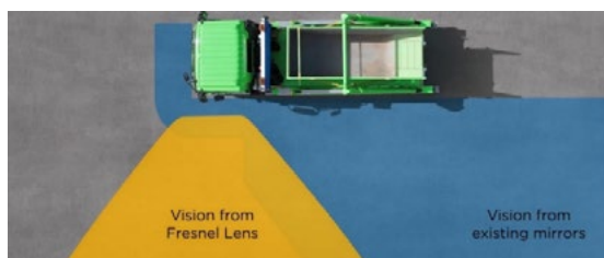
A Fresnel lens can illuminate a truck's passenger-side blind spots.
