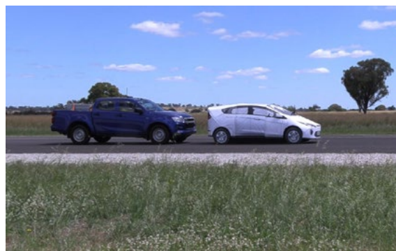
Testing of a vehicle's Autonomous Emergency Brake system while approaching behind a slower-moving vehicle target, at the Future Mobility Testing and Research Centre.
