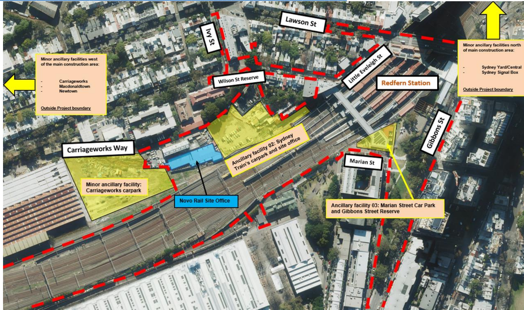
Figure 6-2 Site layout plan – ancillary work locations/laydown areas and rail corridor access points
