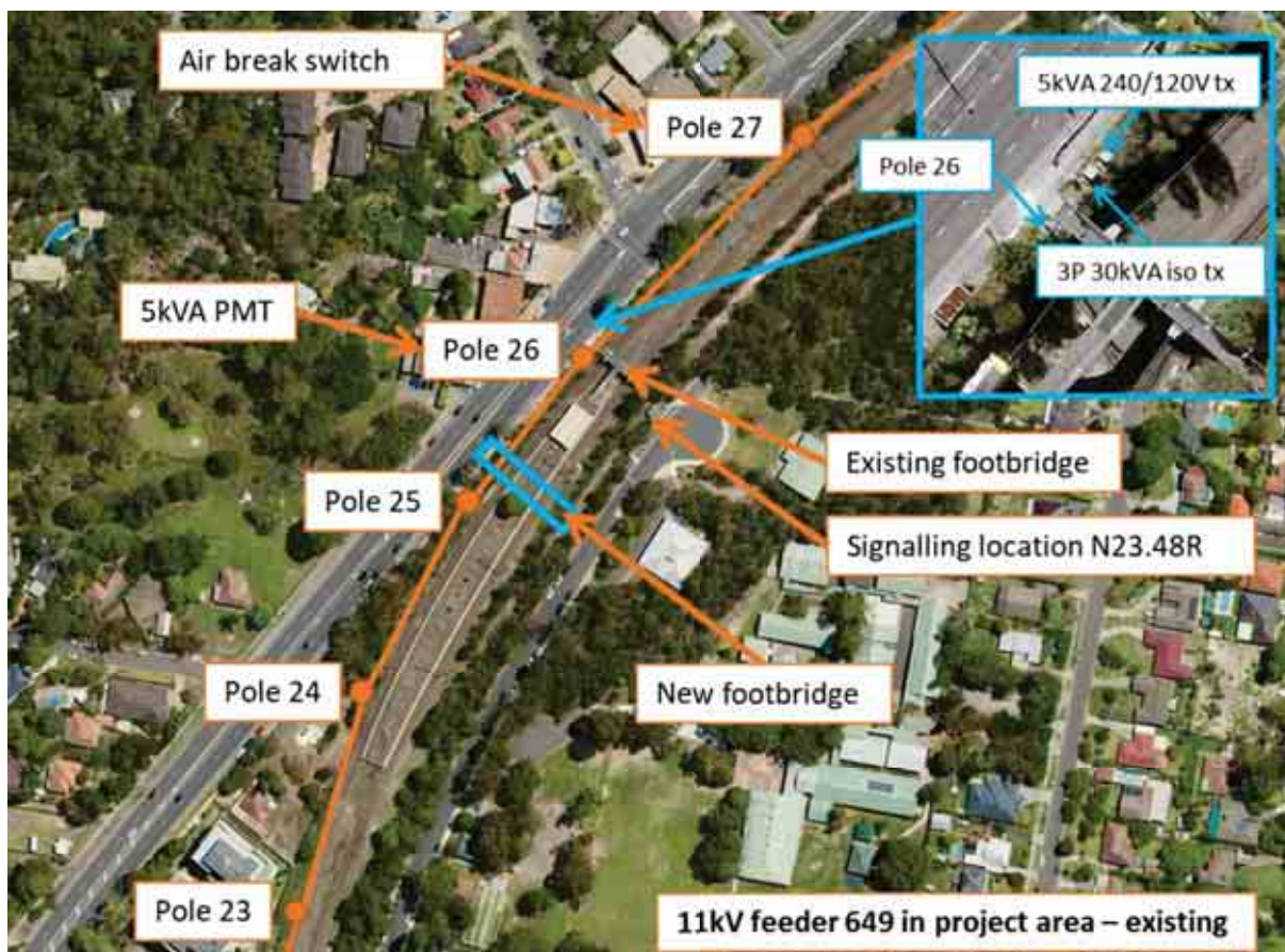
Figure 1: Existing 11kV feeder 649 arrangement
