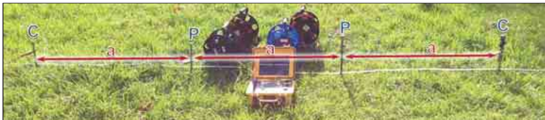
Figure 4: Wenner 4 Pin Method
