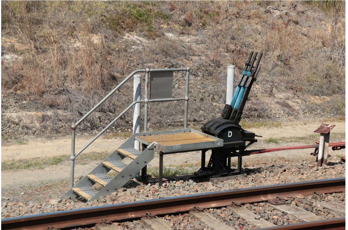
Figure 4-2: 1930s ground frame, installed in location c.1980s. See also Figure 3-8
