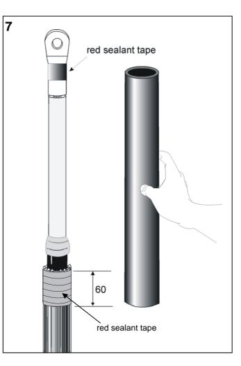
Shrink the tubing down starting at the insulation screen cut. Heat the area well but avoid scorching the surface. Continue shrinking towards the cable lug. Finally shrink down the bottom end of the tubing.
