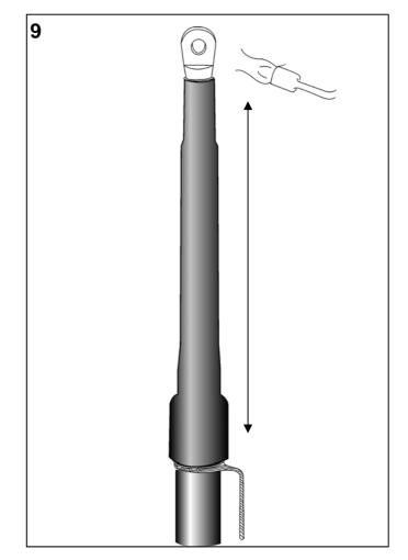
Gather the screen wires together on each core to form a separate earth lead.
