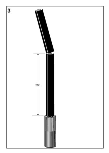
Thoroughly remove the insulation screen to 40mm above the inner sheath cutback.
