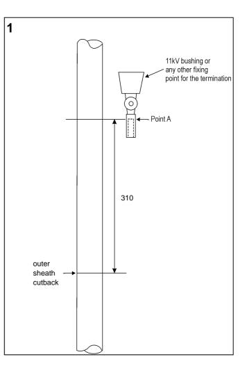
Remove the outer layer of the composite sheath for 310mm.
