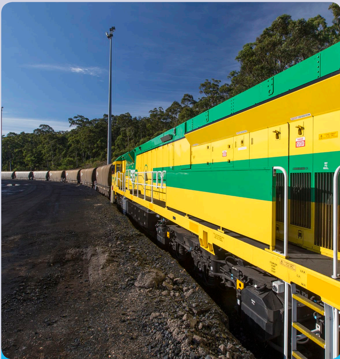
This locomotive is part of a train set hauling coal for Centennial and entered service in 2012. The C44aci model meets the NSW EPA noise emission standards for new or substantially modified locomotives. Currently there is no corresponding EPA standard for particulate or air emissions from locomotives however these new locomotives meet the company's self imposed targets.
