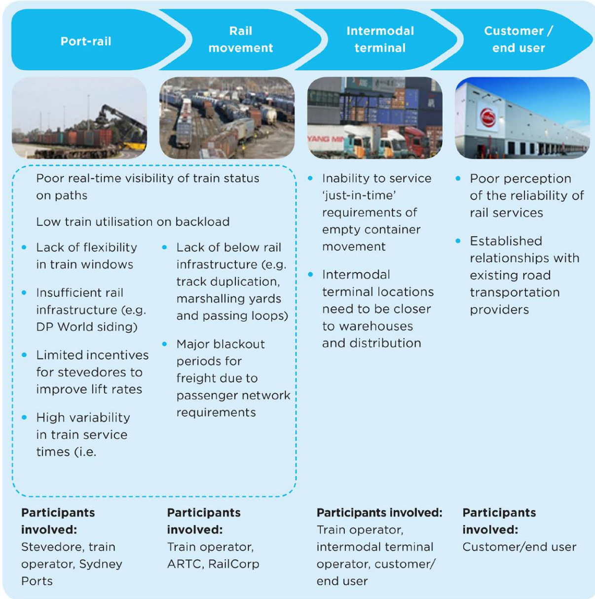
Figure 24 Barriers to efficiency in the movement of containers by rail to and from Port Botany
