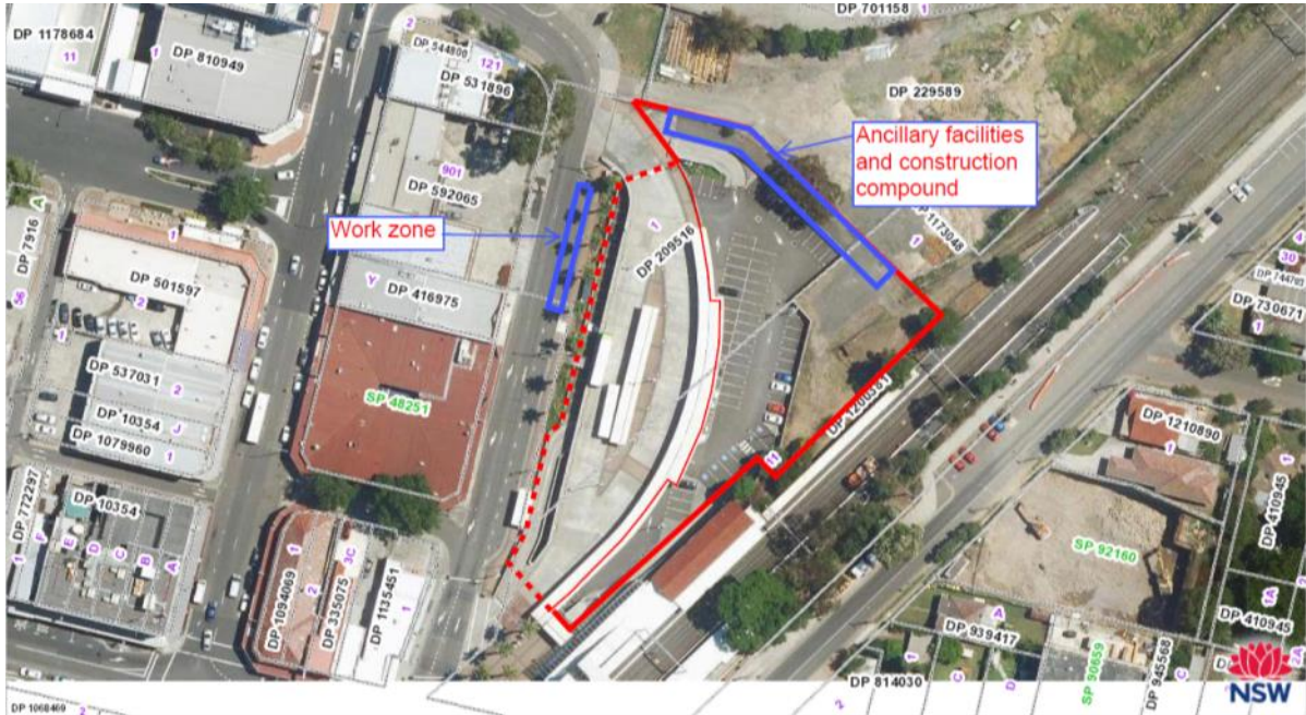
Figure 13 Site 1 Construction Site Footprint, showing indicative location of the site compound and works zone (TfNSW, 2016)
