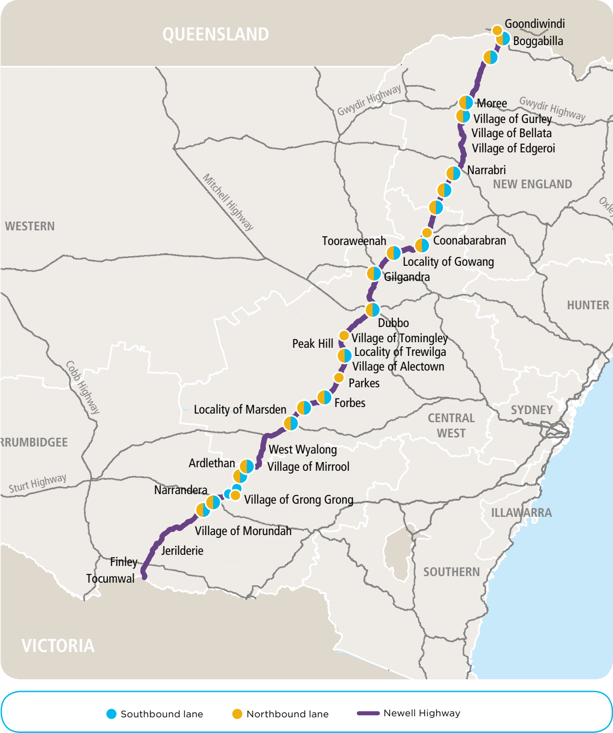
Figure 4.20 Locations where lane widths are less than 3.25 metres
