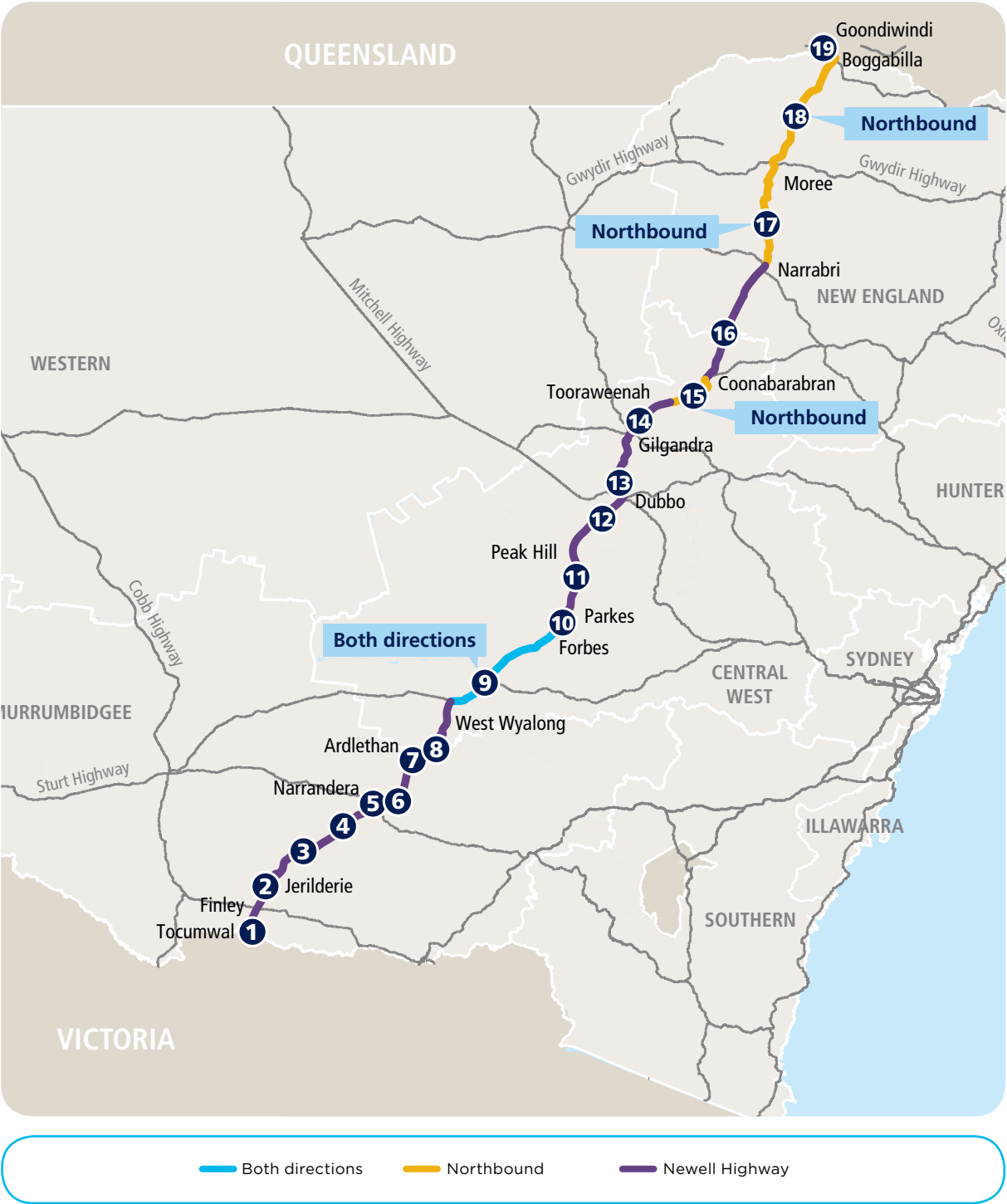
Figure 4.12 Sections of the Newell Highway that do not meet the network planning target for the provision of overtaking lanes
