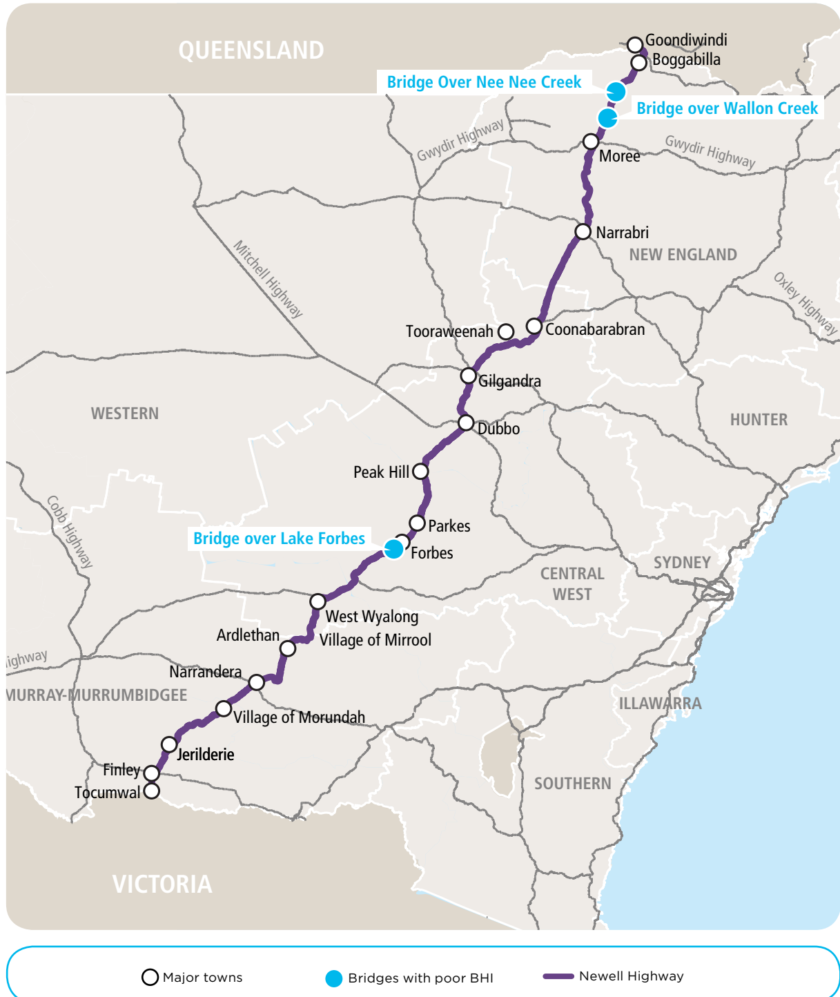
Figure 4.22 Locations of bridges with poor Bridge Health Index (BHI)
