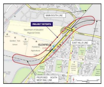
Given the size of the engineering tasks required to achieve the connection, there is also an opportunity to remodel the East Hills connection to remove the existing flat junction and associated restrictions, thereby improving the capacity at Glenfield Junction.
