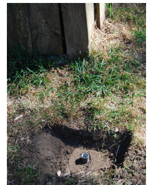
Galvanised Iron Pipe references boundary corner
