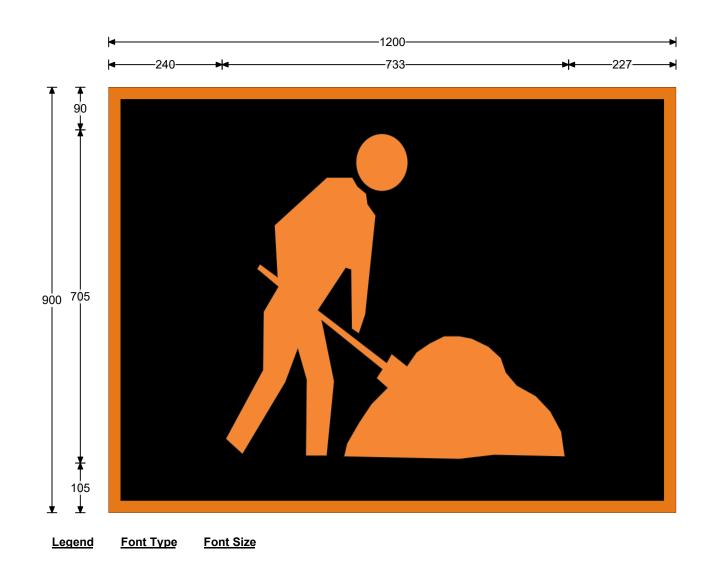
LED details are indicative only. Should be developed in accordance with standard display requirements in AS4852 & Transport for NSW specification TSI-SP-008. For performance and operating instructions refer to Transport NSW ITS Helpdesk Email:-ITSHelpdesk@transport.nsw.gov.au
