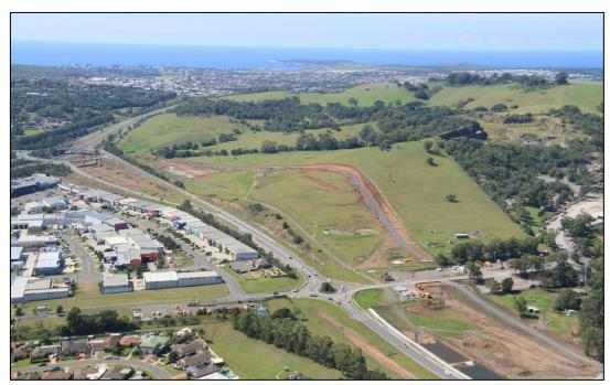
**Figure 1:** Aerial view of Cut 5 of the Project during April 2019 (looking towards the southeast). Initial works in this area focussed on the installation of drainage controls.
