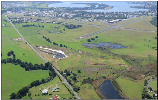
**Figure 2:** Aerial view of Fill 8 of the Project during April 2019 (looking towards the northeast). Project sustainability initiatives have been trialled at this location via the use of imported coal wash/rejects as fill material.
