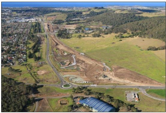
**Figure 1:** Aerial view of the southern portion of the project corridor during late June 2019. Bulk earthworks associated with the new alignment and new East-West link road are visible on the central portion of this photograph with the Green Meadows detention basin and Cut 5 work areas beyond.
