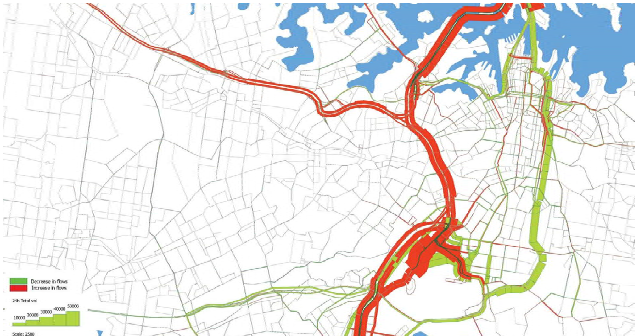
Figure 24 2033 average weekday traffic flows, with versus without Sydney Gateway, M6 Stage 1, Western Harbour Tunnel and Beaches Link (M4-M5 Link EIS, Roads and Maritime, 2017)
