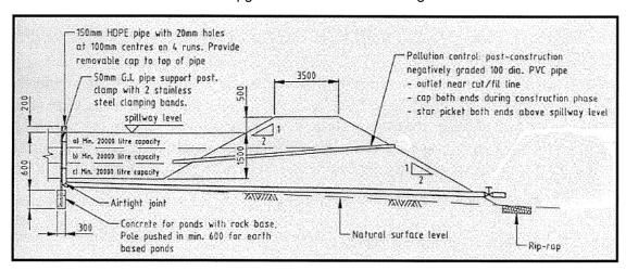
Figure 3 Cross section of a sediment pond incorporating insoluble pollutant control (source: NSW RTA)
