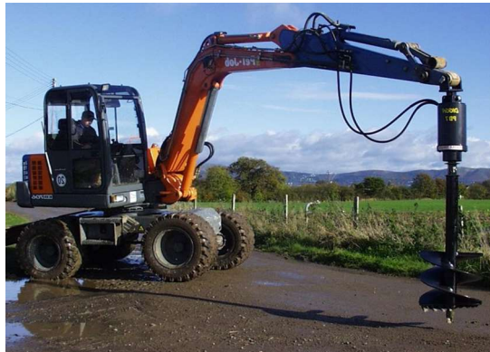
Figure 5. Example - wheeled excavator with auger attachment for extended reach.
