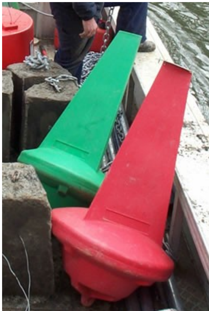
Above: Example of Port and Starboard Lateral Buoys that can be used.
