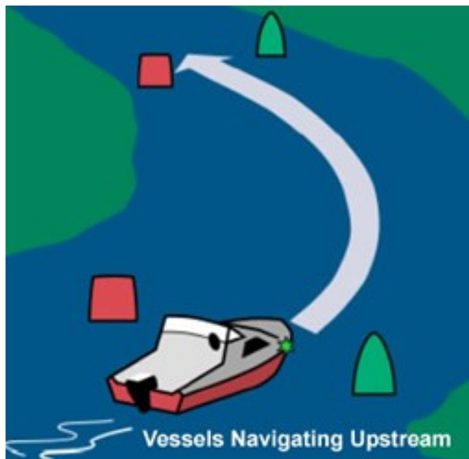
Above: Example of how Port and Starboard Lateral Buoys are used to create a navigable channel.
