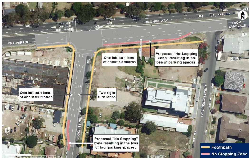
Map showing proposed improvements and parking changes on Bigge Street and the Hume Highway
