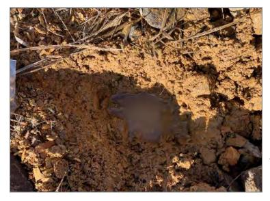
AOI – 1 – Weathered, saturated orange silts generated from cutting wall under ballast. Taken from the eastern side of a railway switch.
