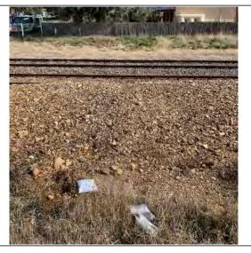
T3-E2 – Sampling atop the railway cutting. Sandy gravelly fill similar to sub-ballast fill.
