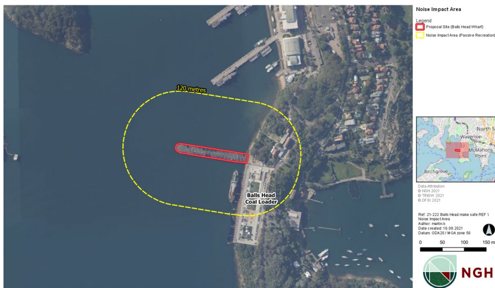
Map showing anticipated noise impact area for the make safe and retrieval work for the Coal Loader Wharf
