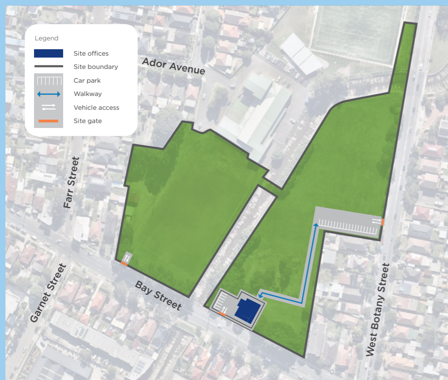
Construction site layout at Ador Park Precinct and McCarthy Reserve
