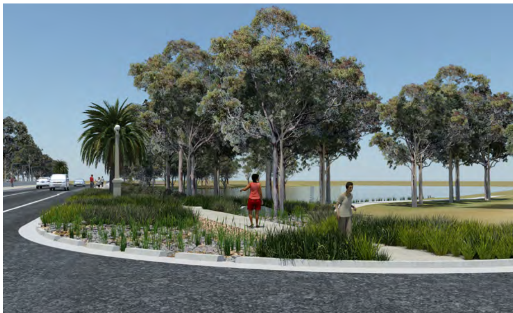
Figure 4.30 This view captures the area where a slotted kerb is used to capture rainwater run off and feeding it into a rock mulched area /infiltration area where the water is cleaned and slowed down, prior to it discharging into the lake
