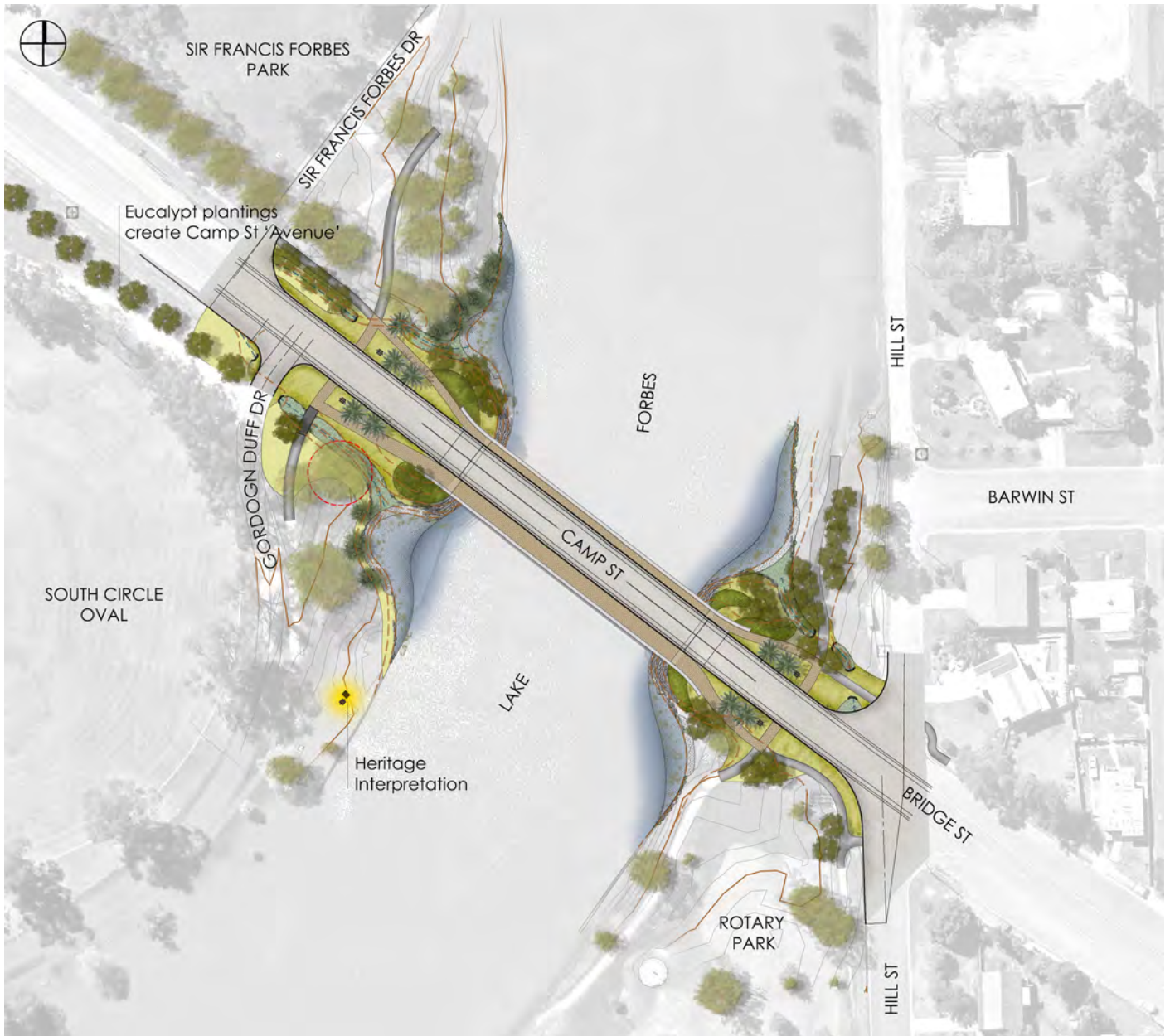
Figure 4.17 The proposed landscape design incorporates water sensitive design elements that soften the lake edge by curving the lake/land interface more to create more natural, organic shapes as well as improving water quality.
