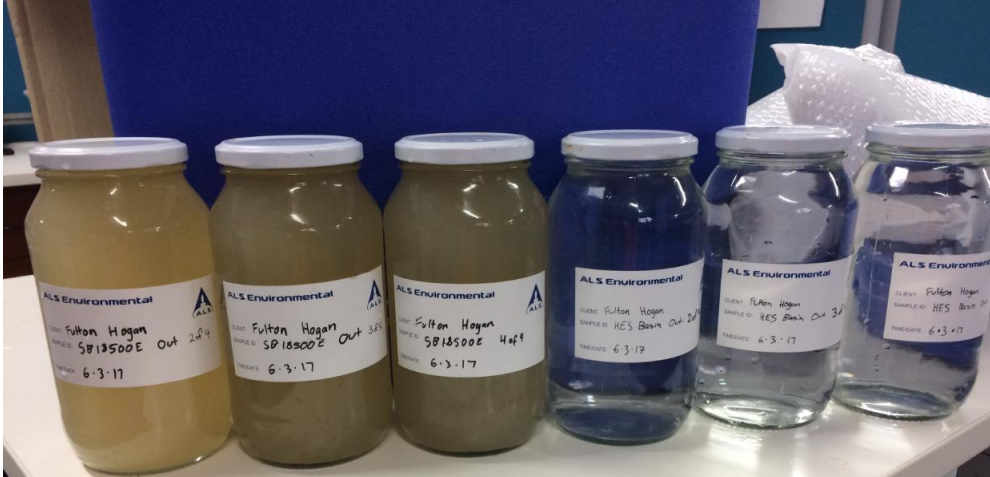
Figure 4-1: From left to right: Samples taken from batch basin vs HES Basin after rain event
