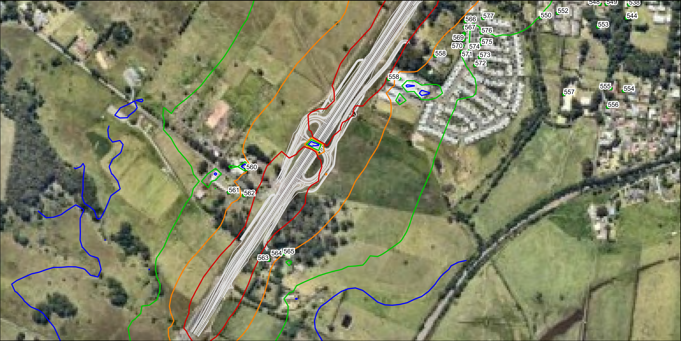
FOXGROUND BERRY BYPASS FIGURE 16 Predicted night-time road traffic noise levels - 2027 SECTION 4: South of Berry
