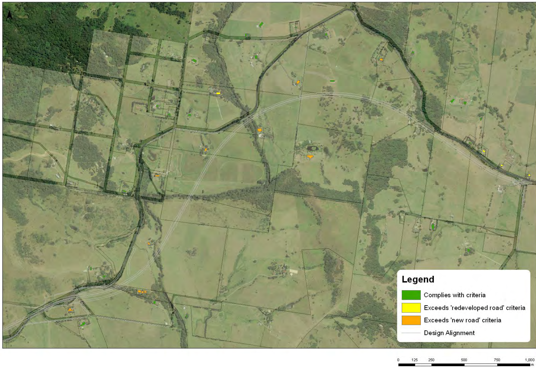
Figure 4-1: Receivers predicted to exceed criteria in areas from Toolijooa Road interchange to just east of the Austral Park Road interchange
