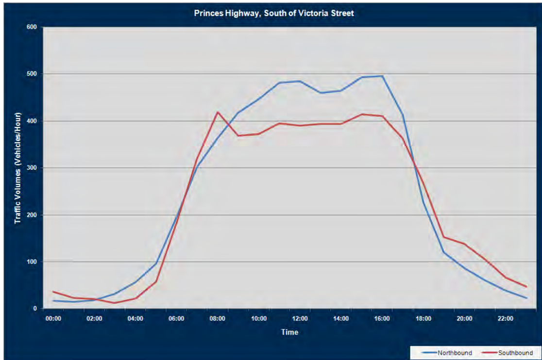
Figure 2.8: Average daily traffic profile: Princes Highway south of Victoria Street (2011) (Source: AECOM, based on RMS Southern Region Traffic Survey Data)
