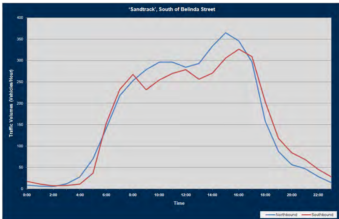
Figure 2.9: Average daily traffic profile: 'Sandtrack', south of Belinda Street (2009) (Source: AECOM, based on RMS Southern Region Traffic Survey Data)
