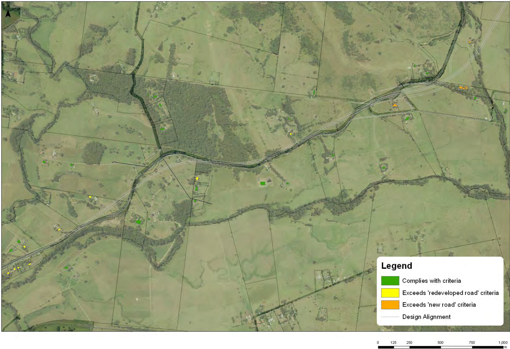
Figure 4-2: Receivers predicted to exceed criteria in areas between Austral Park Road interchange and Tindalls Lane interchange
