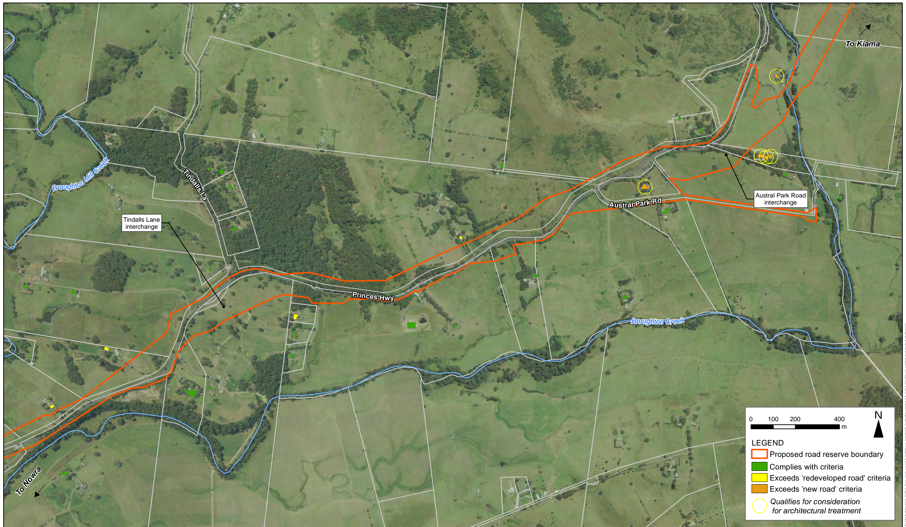
Figure 7-5 Receivers predicted to exceed criteria in areas between Austral Park Road interchange and Tindalls Lane interchange
