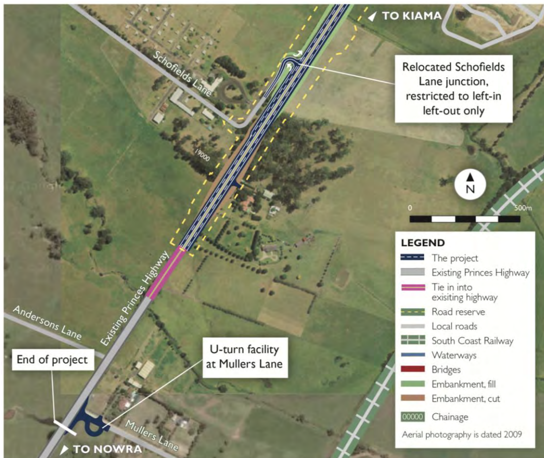
Figure 4-14 Schofields Lane junction
