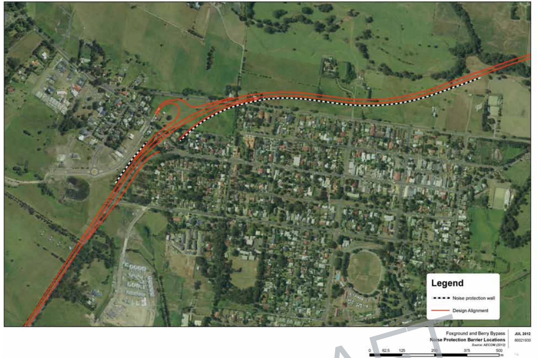
Figure 7: Acoustic analysis - noise barrier locations.
