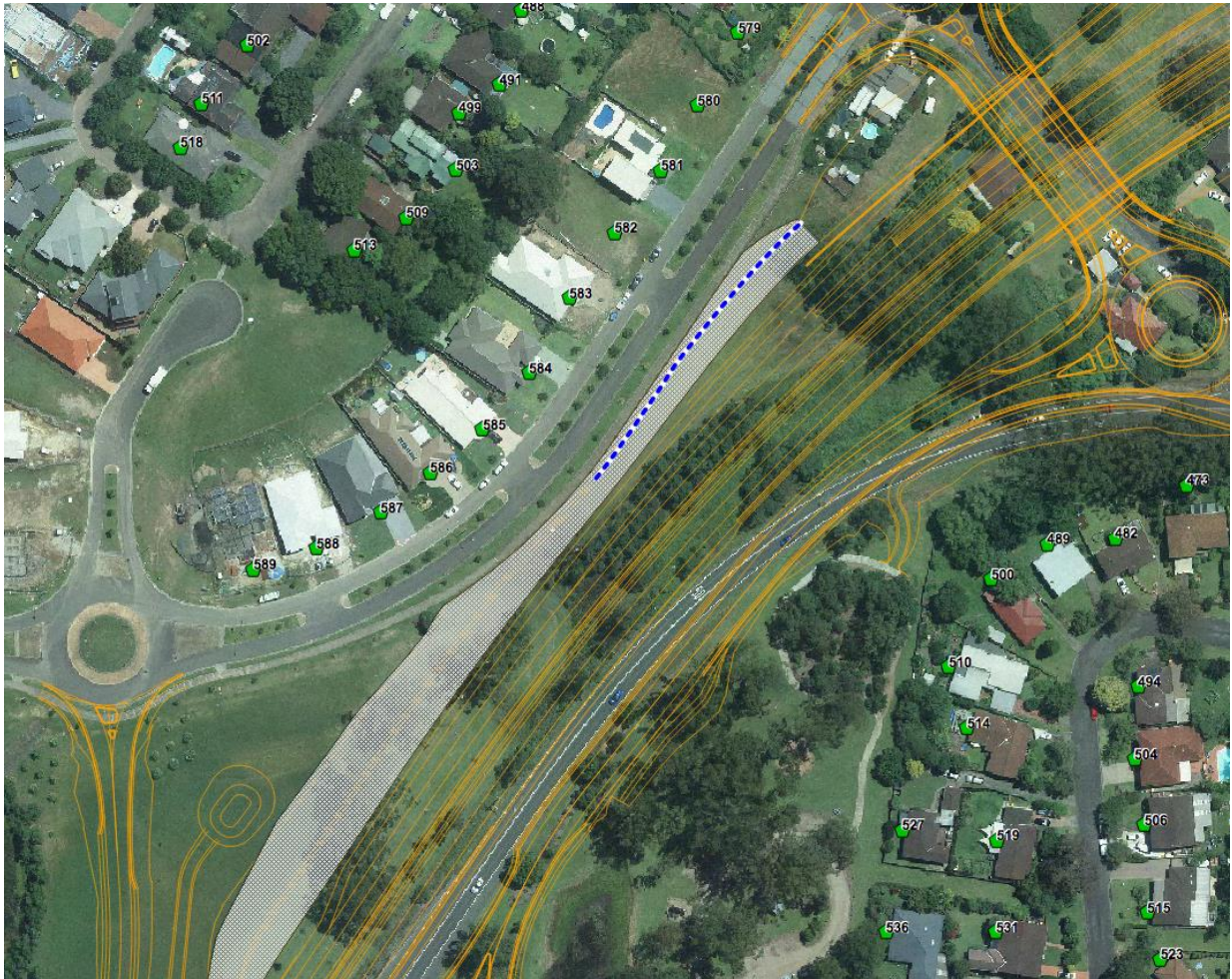
Figure 6-4: Huntingdale Park Road noise mound (shaded) and 800 mm high barrier (shown in blue).
