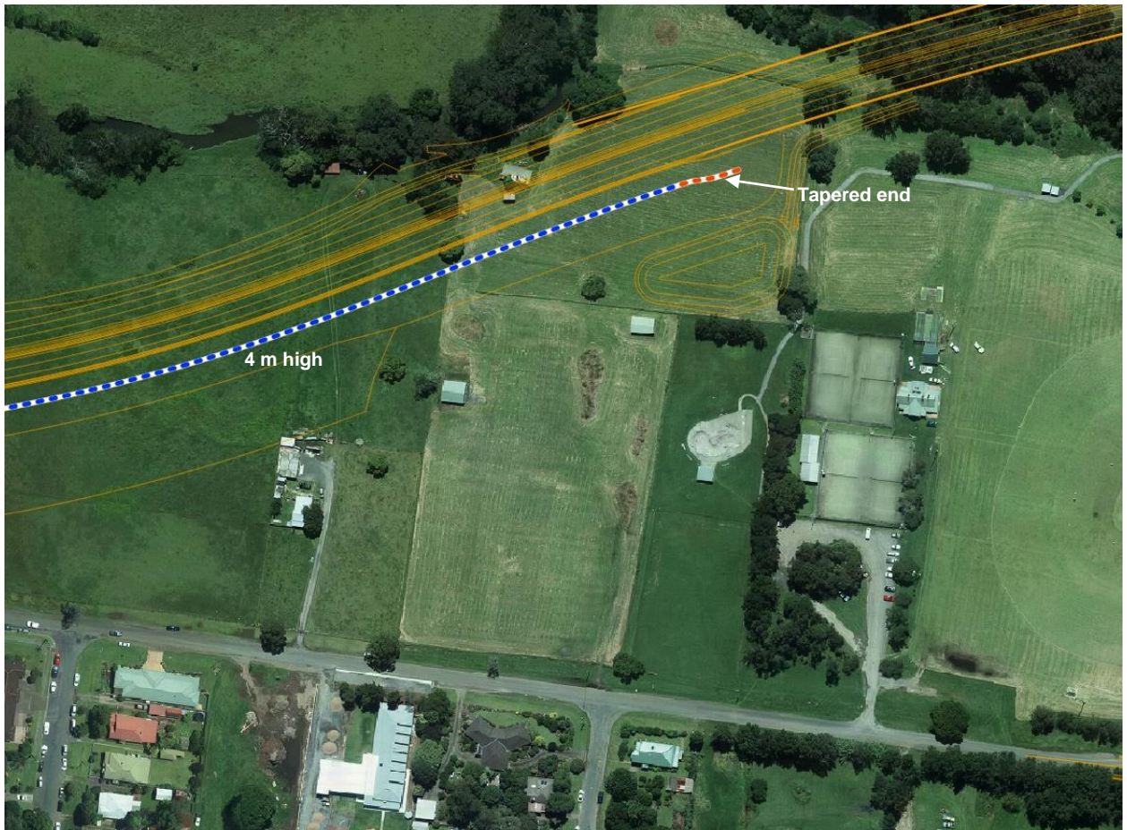
Figure 6-2: Eastern end of barrier NB01, orange section indicating length where noise mound may be tapered as an end treatment.
