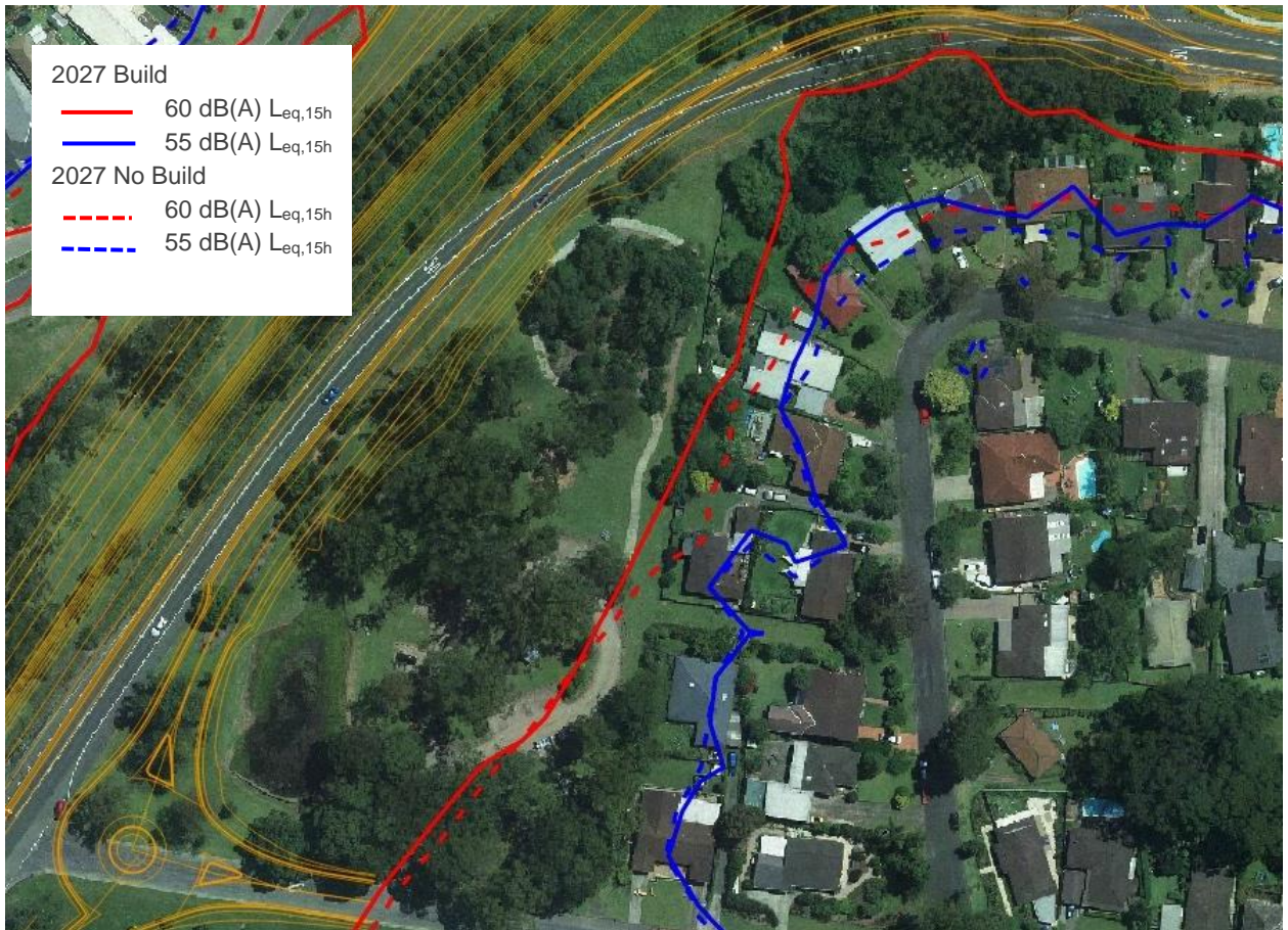
Figure 6-5: Predicted 2027 'Build' and 'No Build' L_{eq,15h} traffic noise levels at Mark Radium Park
