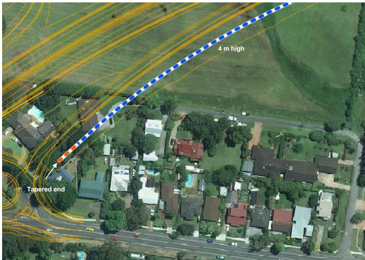
Figure 6-3: Western end of barrier NB01, orange section indicating length where noise mound may be tapered as an end treatment.
