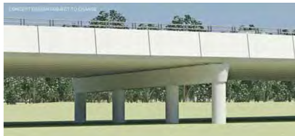
Circular columns with integrated headstock
