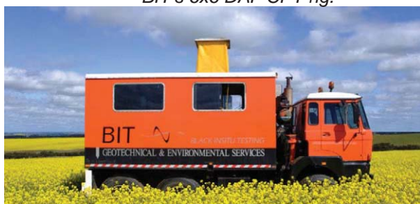
BIT's 6x6 DAF CPT rig.
