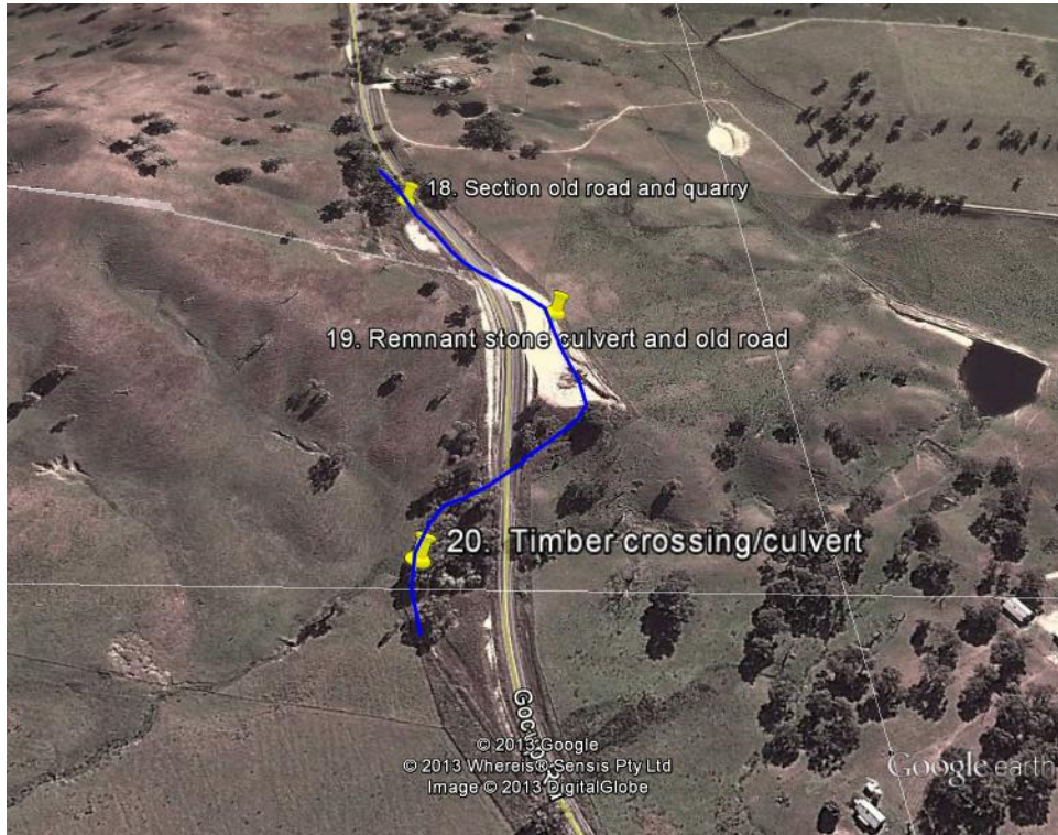
Figure 4.55: Location of the timber crossing/culvert #20 on the abandoned road alignment (shown in blue) and in relation to the present alignment of the Gocup Road.
