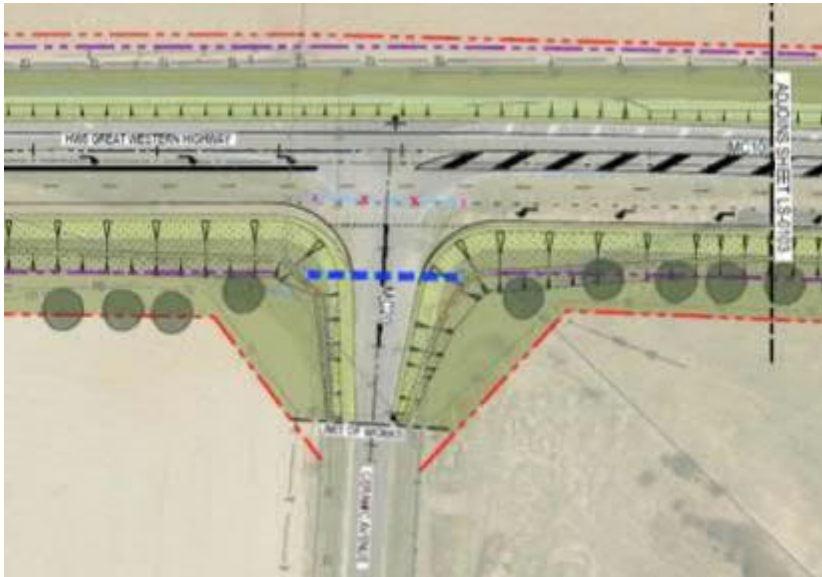
Figure 4-10 Proposed intersection at Ceramic Avenue (extract from Urban Design and Landscape Plans in Appendix B)
