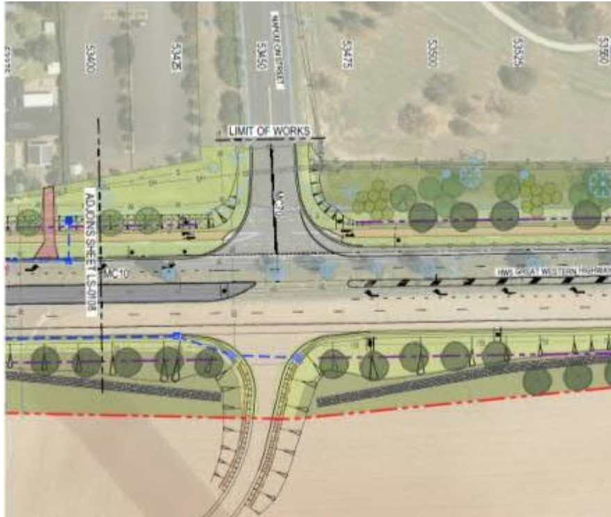
Figure 4-5 Proposed intersection at Napoleon Street (extract from Urban Design and Landscape Plans in Appendix B)
