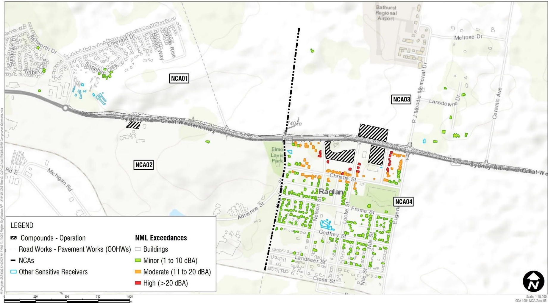
Figure 9 Predicted Impacts 'W.10 – Compound – Operation' (Night-time)
