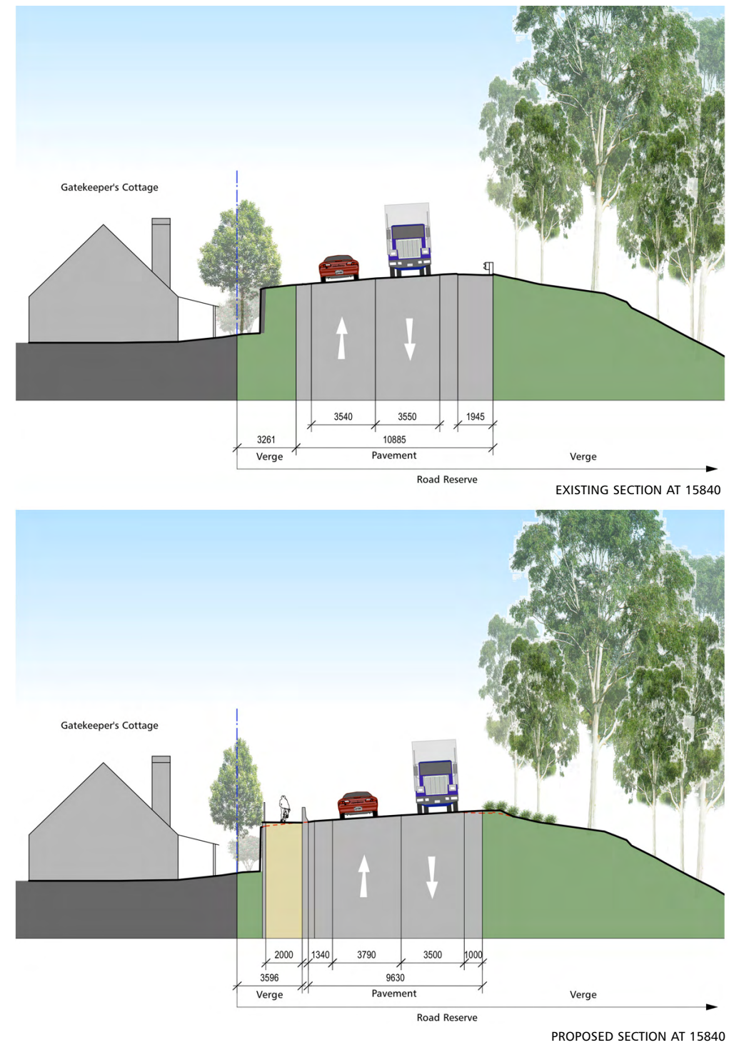
Figure 4.3: Section B at chainage 15840.
