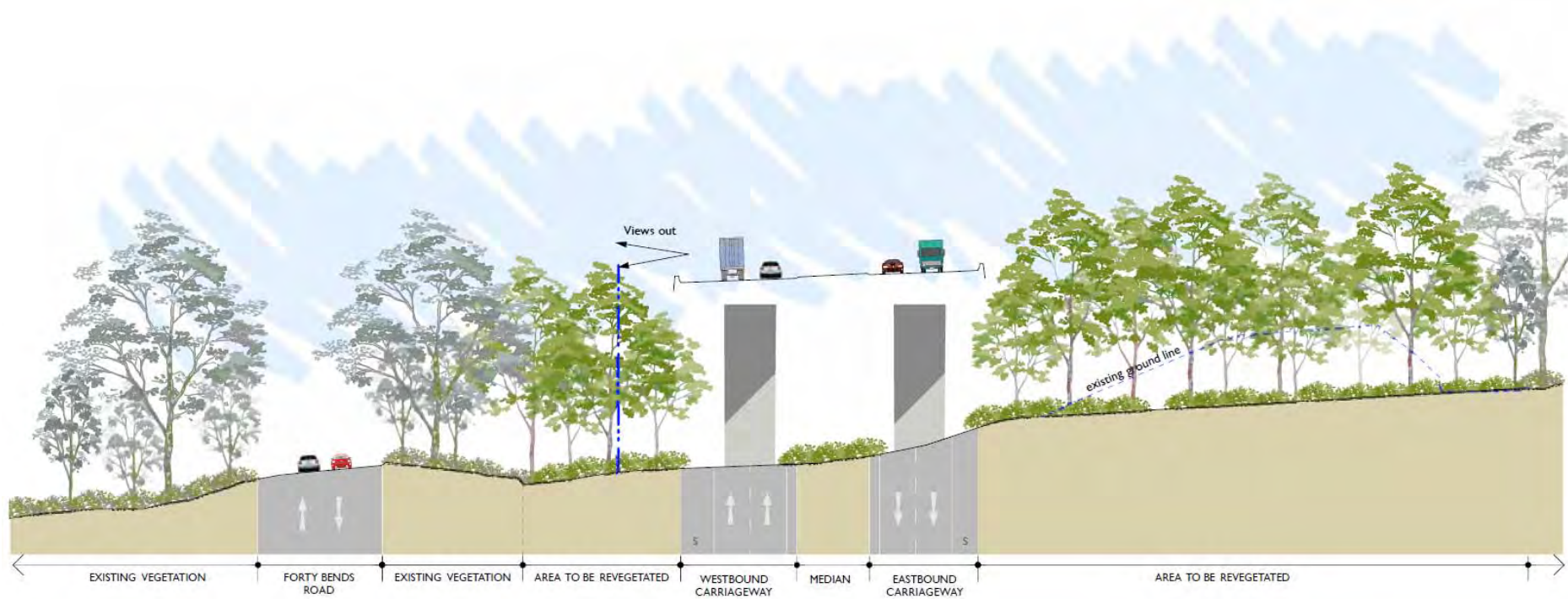
Figure 3-7: Indicative cross section of the Whites Creek bridge (Chainage 31700)
