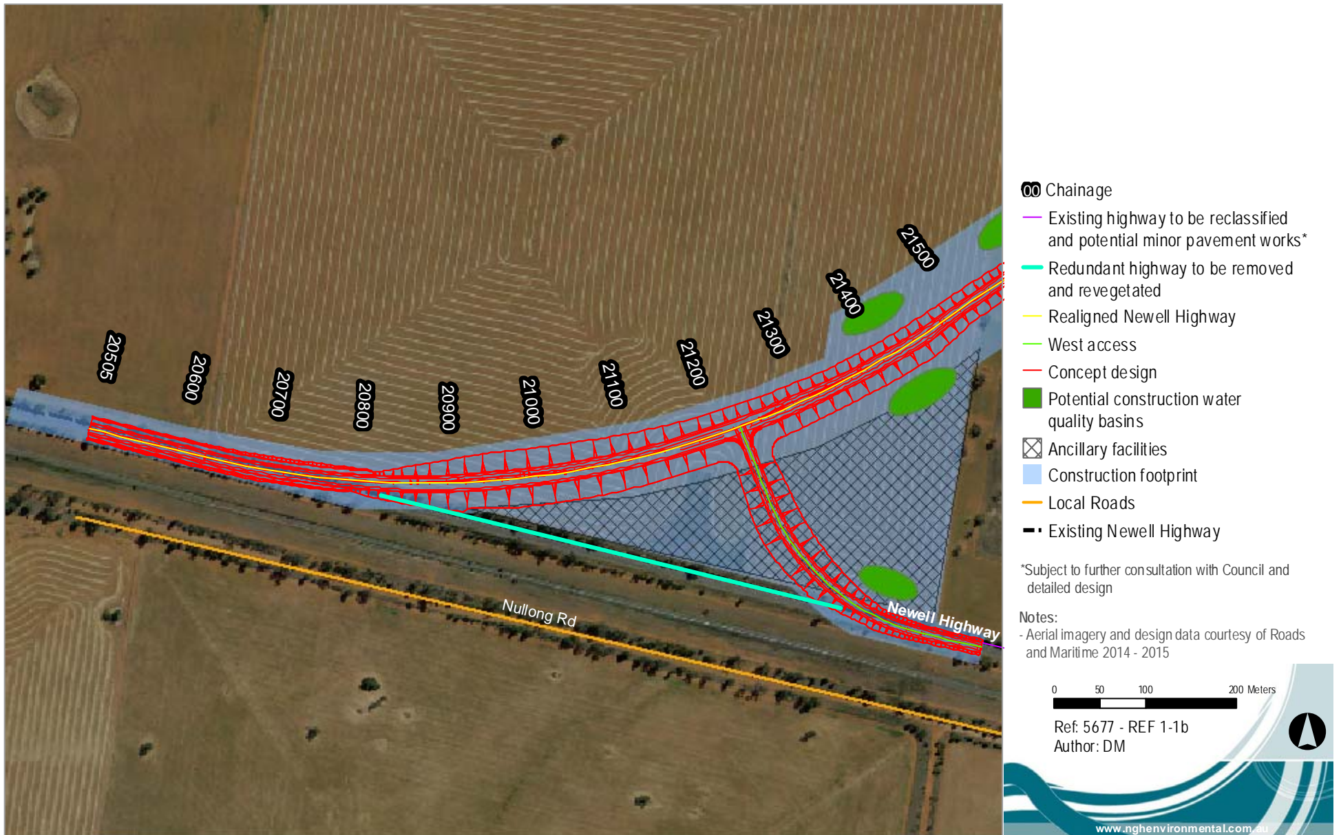
Figure 1-2c: Western access detail
