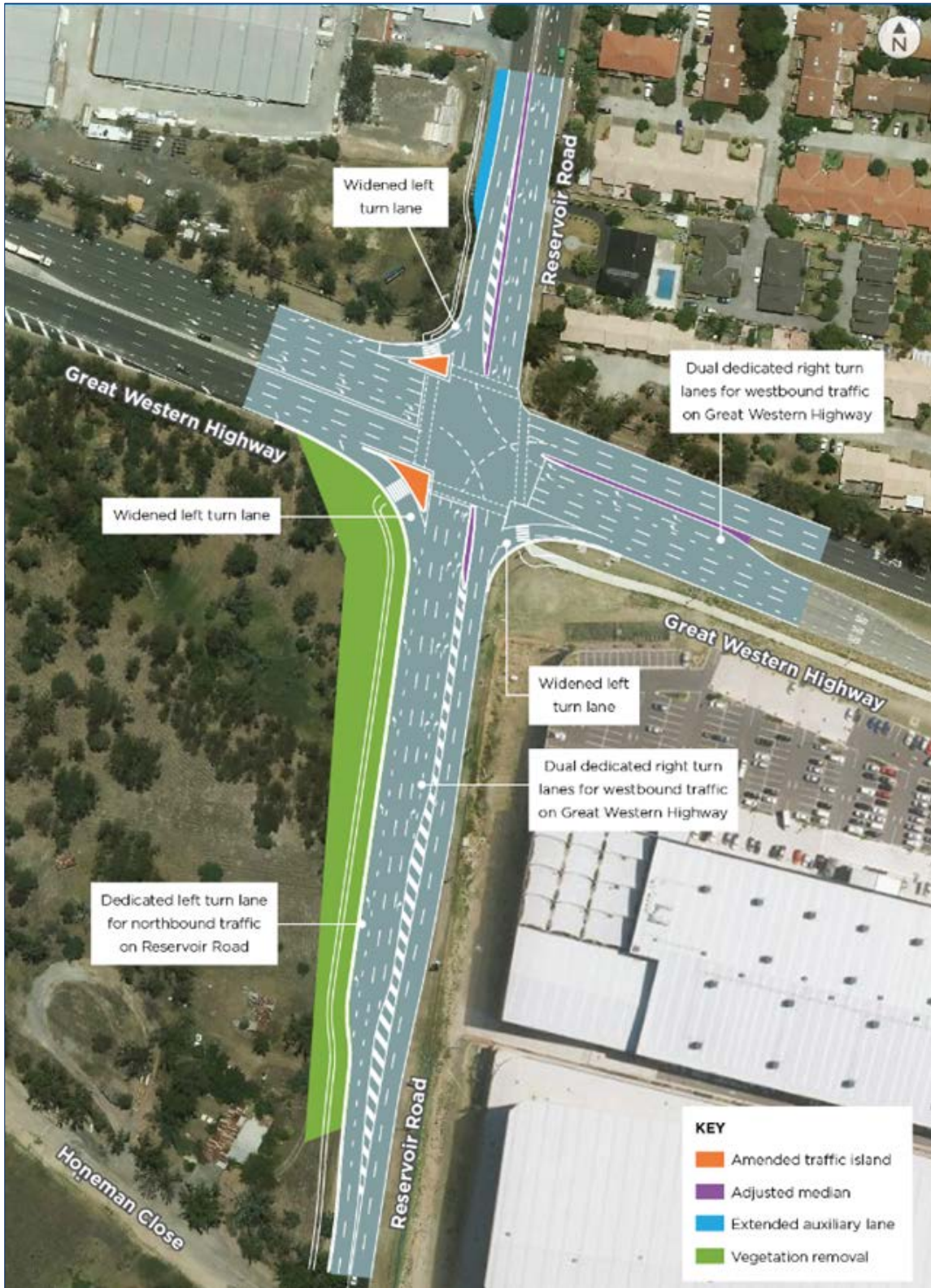
Figure 1: Proposed improvements at the intersection of the Great Western Highway and Reservoir Road, Blacktown
