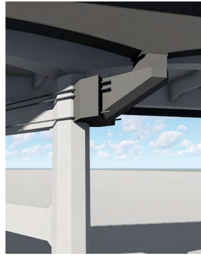
Figure 5.4 Indicative 3D detail study of the bolt connections. The steel rods avoid the existing structure to ensure its integrity.
