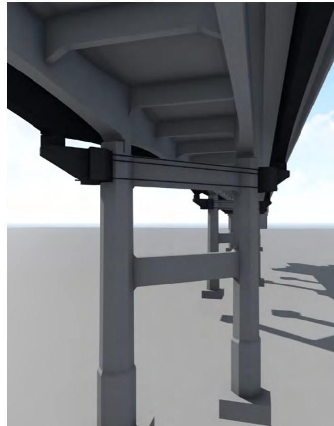
Figure 5.3 Indicative 3D study of the pier and new headstock extension. Steel rods would be used to clamp the two knuckles to the existing pier.
