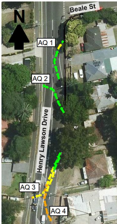
Figure 3.14 - Aquaplaning flow paths near Beale Street intersection
