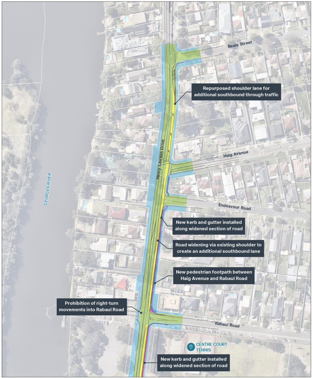
PROPOSAL AREA - KEY FEATURES AND WORKS EXTENT RABAUL ROAD TO BEALE ST
