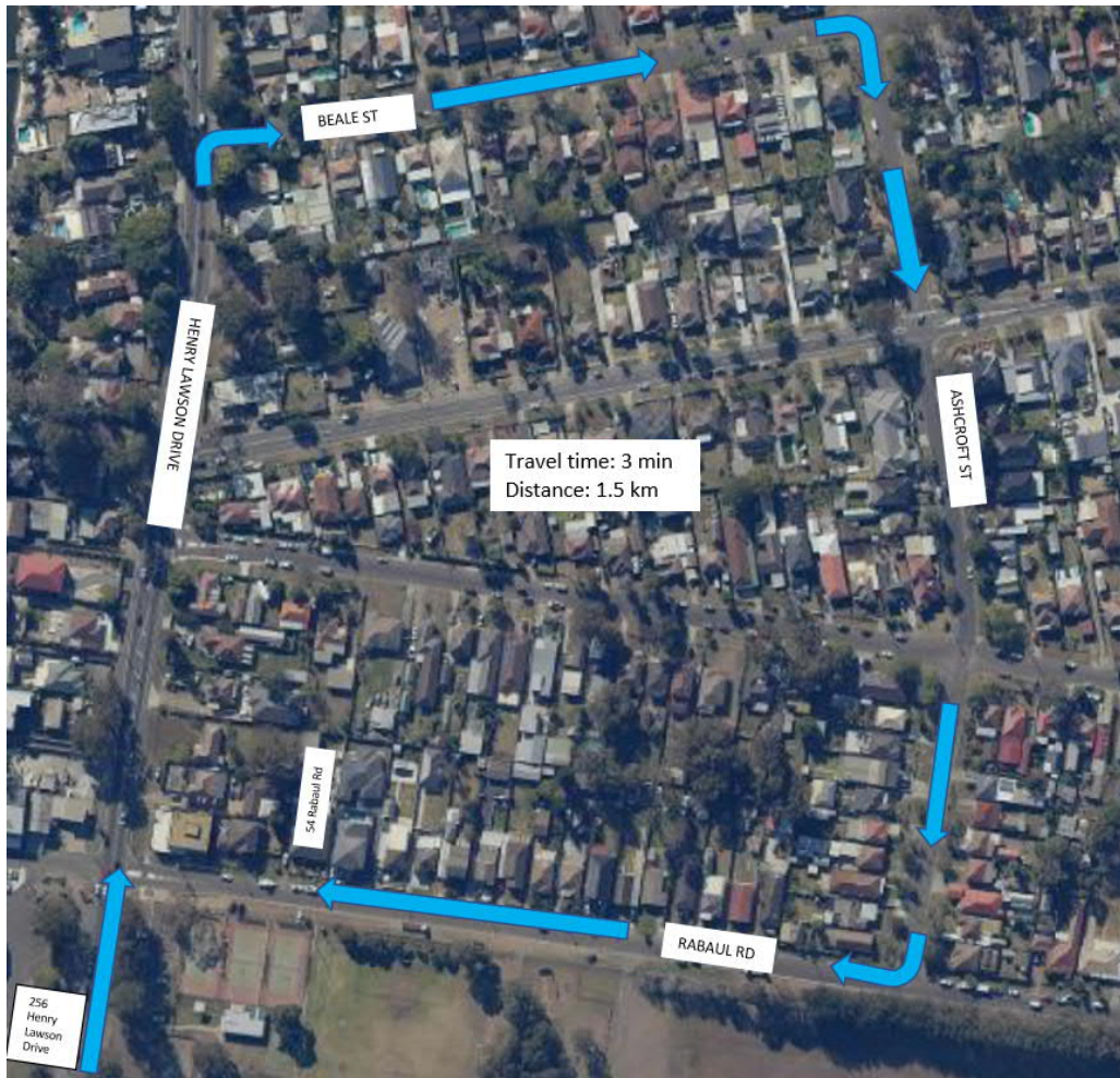
Figure 4: Right turn ban at Rabaul Road, vehicles taking right at Beale Street and Ashcroft Street to access Rabaul Road (image: six maps)
