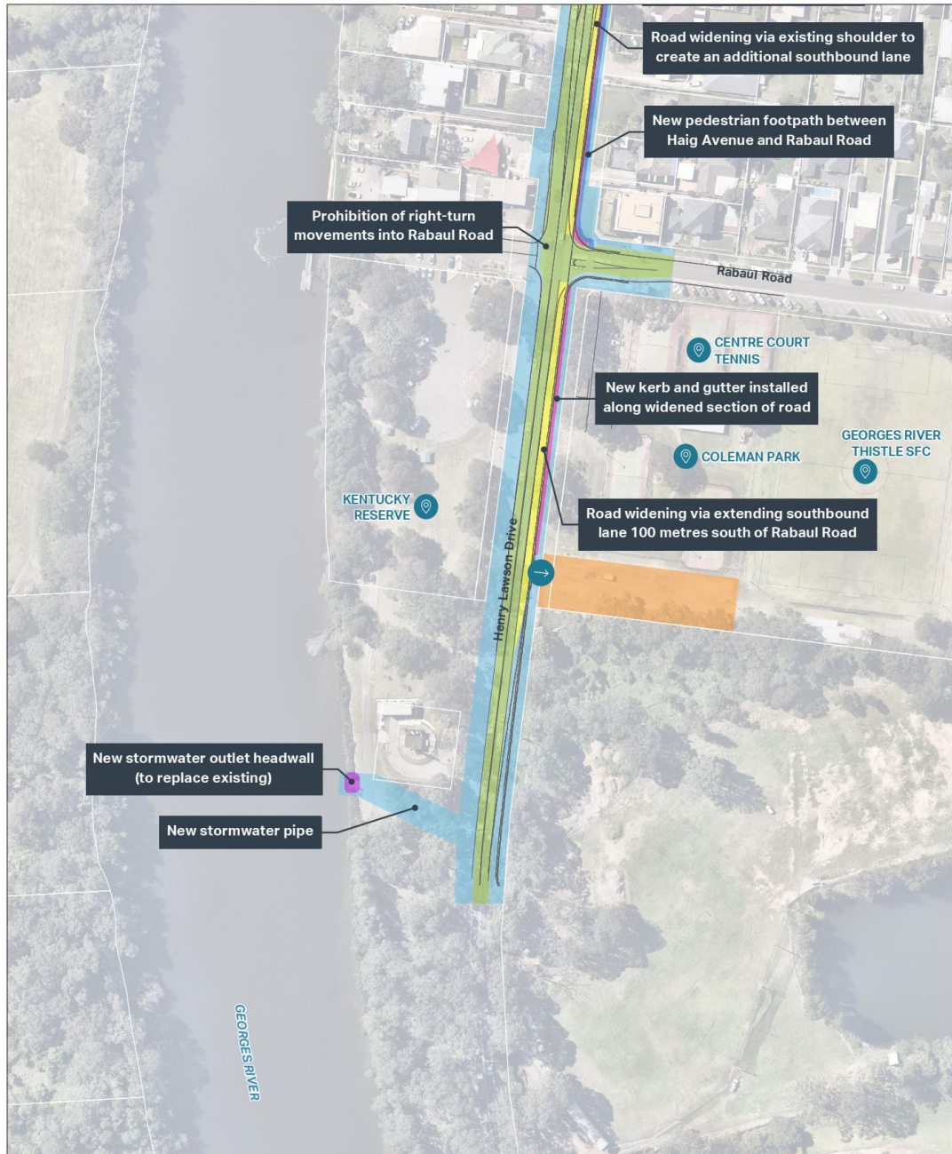
PROPOSAL AREA - KEY FEATURES AND WORKS EXTENT 256 HENRY LAWSON DRIVE TO RABAUL ROAD
