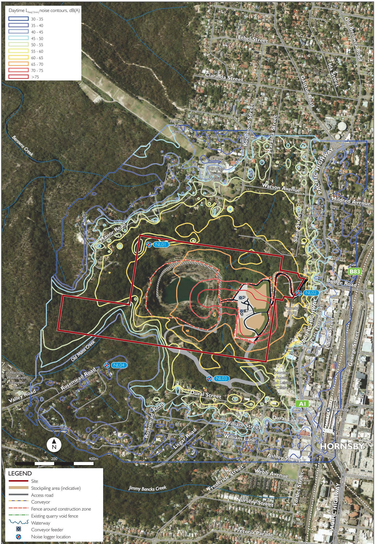
Appendix D Figure 7 Conveyor construction noise contours (cumulative)
